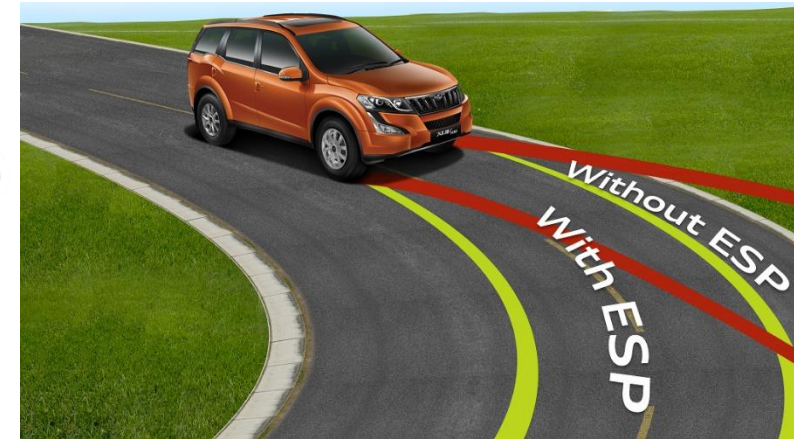
Electronic Stability Program (ESP)
